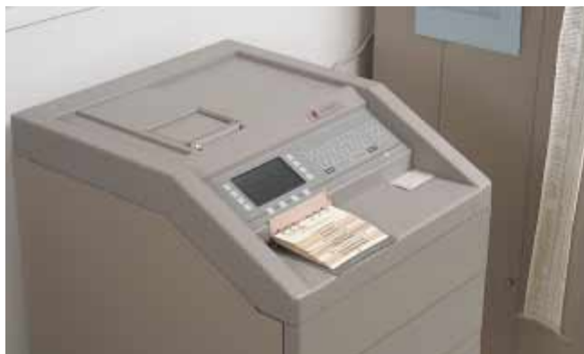
Figure 29-6 Computer-controlled Dispensing System
