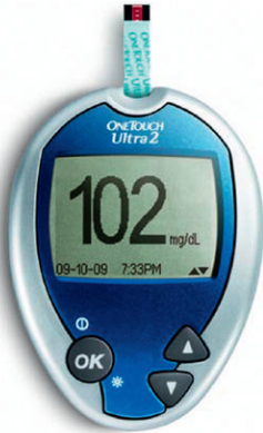
Fig. 9-1 Blood glucose monitor. (Courtesy LifeScan, Milpitas, CA.)
