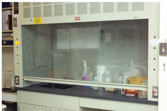
FIGURE 5-1 Fume hood used for toxic hazards found in the laboratory. Source: Delmar/Cengage Learning.
