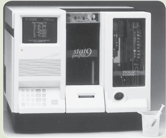
FIGURE 14-5 Nova CCX analyzer that uses ion-selective electrode technology for a variety of analyses. Source: Delmar/Cengage Learning.
