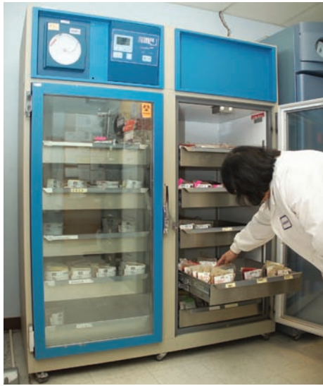
FIGURE 7-8 Blood bank refrigerator designed to store units of blood according to group and type, and special units for patients with unusual blood types or atypical antibodies. Source: Delmar/Cengage Learning.
