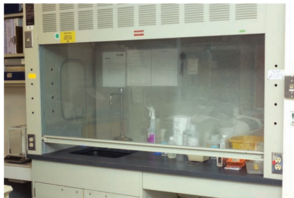
FIGURE 7-13 Fume hood used for working with toxic chemicals that are volatile. Source: Delmar/Cengage Learning.
