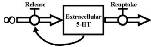
Fig. 2 A “stock and flow” diagram of a control system model of serotonin (5-HT) function. The stock of extracellular serotonin is increased by presynaptic neural activity (i.e., release) and is decreased by serotonin transporter-mediated reuptake. When extracellular levels of serotonin are above some threshold, somatodendritic autoreceptors (serotonin-1A) inhibit neural firing via a feedback mechanism. When presynaptic neural firing is enabled, terminal autoreceptors (serotonin-1B) control the serotonin release amount. The infinity sign represents an infinite reservoir for the production of serotonin
